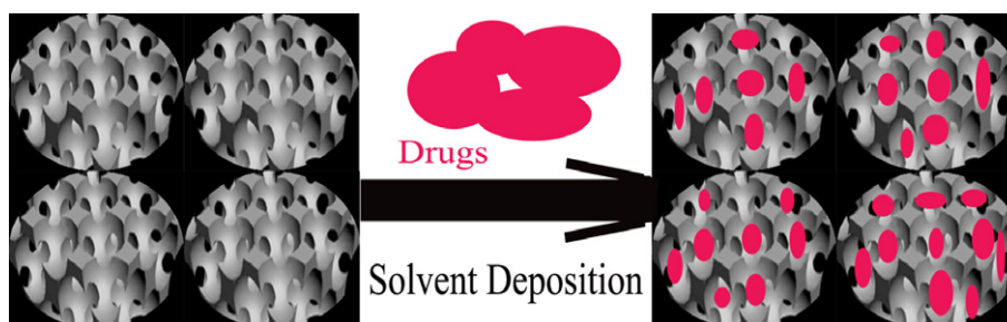
Fig. 2. Schematic representation for incorporation of IMC nanoparticles into 3DOM silica matrix. By solvent deposition method, the original large crystals of IMC can be successfully entrapped into pores of 3DOM silica in the form of nanoparticles, thus allowing for the proper size control of drug particle size. (For interpretation of the references to color in this figure legend, the reader is referred to the web version of this article.)
